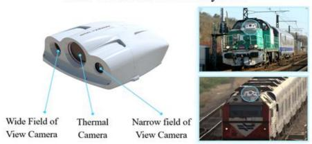
Our railway detection system is designed to discover and warn the train operator about hazards of up to 2,000 meters (1.2 miles) ahead of the train. To detect hazards up to this distance, our railway detection system is dependent on a continuous line of sight that is not obscured by buildings or curves in the track.
